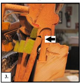
When a bridle strap is missing and the action is returned to the piano the jack (the vertical part shown in the above photo) is prone to jamming up against the underside of the hammer butt.
