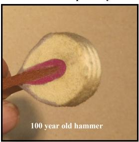
When hammers are new, as in the photo on the above left, the outer surface is rounded smoothly. The striking surface has no indentations. Over time, as the hammer repeatedly strikes the steel strings of the note it is matched with, the metal strings begin to bite into the stiff felt of the hammer. As more and more fibers in the hammer are broken over time, the cuts become deeper. Eventually, the once-smooth hammer takes on the appearance of the hammer on the right.
