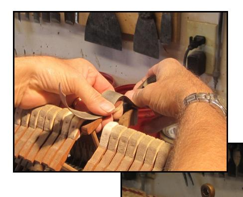
Hammers are shaped by hand sanding with either a sandpaper file or a sandpaper strip, both of which are shown above. The sanding technique involved requires a great deal of practice to perfect and should only be performed by a professional.
