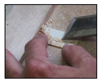
Next, any keytop which has been inexpertly glued to the keystick in the past must be removed and prepared properly. Many times an instrument will have ivories which are poorly glued so that discolorations show through the translucent ivory. The only way to fix this problem is to remove the keytop and scrape the old adhesive off completely, starting over with a proper job of gluing.
