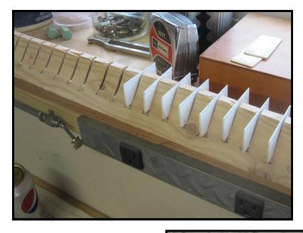
In situations where keytops are loose to the point where they are popping off unexpectedly, the only real solution is to remove them all (usually both heads and tails) and reglue with proper methods that will ensure they stay put in the future. This is one potential aspect of the job which would add a great deal of shop time to the job.
