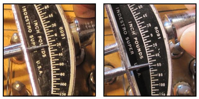
The above photos show torque reading measurements done on the same tuning pin before and after treatment was administered. In the photo on the left, the untreated pin measures just under 20 inch pounds of torque. After a single treatment the pin measures a much better reading of 55 inch pounds of torque.
