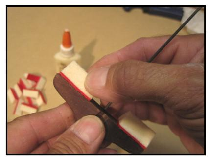
Once the damper heads and guide wires have been attended to, new damper felts will be glued in place, usually at the piano. High quality, precut damper felts are available for many grands. At other times, felt may be cut from strips so that the length of the dampers is precisely fitted to the damper heads.
