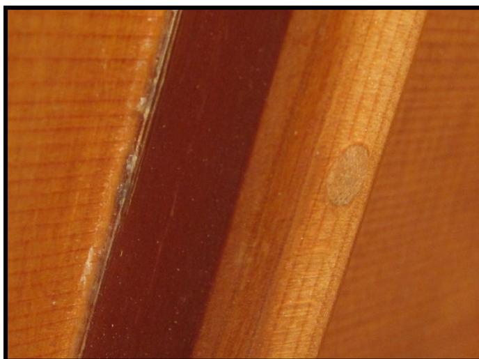
With the ribs glued firmly back into place, the soundboard of your piano will once again perform as intended.
