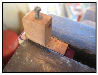
To remove the old dampers, each damper is removed individually from the action along with a part known as the "damper block." Most times the damper block will be reused, with only the damper felt (and possibly its wood backing) replaced. Here, an individual damper assembly is placed in a vise so that the damper block may be removed to be reused.
