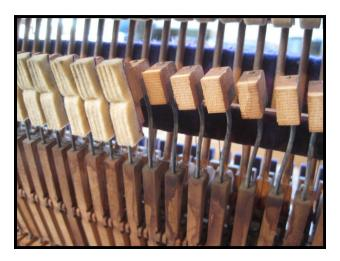
As the damper felts are removed, the damper blocks are returned to the same position they came from in the action.
