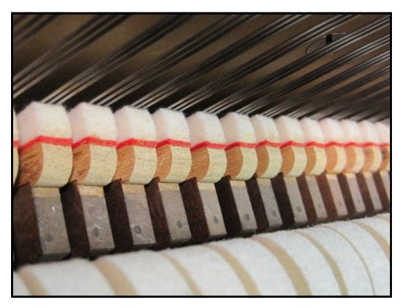
A new set of treble dampers installed and ready to quiet things down when needed.
