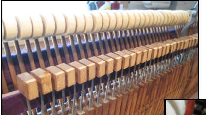
Once all the dampers have been removed, and the dampers blocks have been reinstalled, it is time to return the action to the piano.
