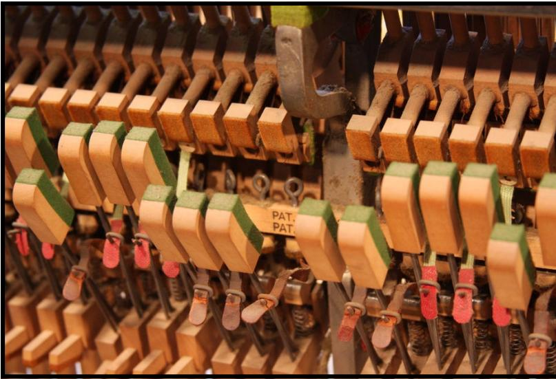
One example of parts which commonly needs to be replaced on a vintage upright piano are the bridle straps, shown in the photo to the left. These straps are essential for holding the bottom of the action up when it is removed from the piano for servicing.
