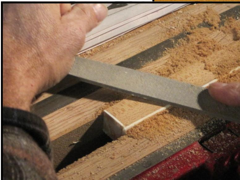
Original ivory in good condition on a vintage upright piano is a definite plus. A few chipped keys may oftentimes be replaced or repaired. In cases where the old keys are badly worn, however, installing a new set of keytops (shown being fitted to the keysticks) will benefit the appearance of the piano.
