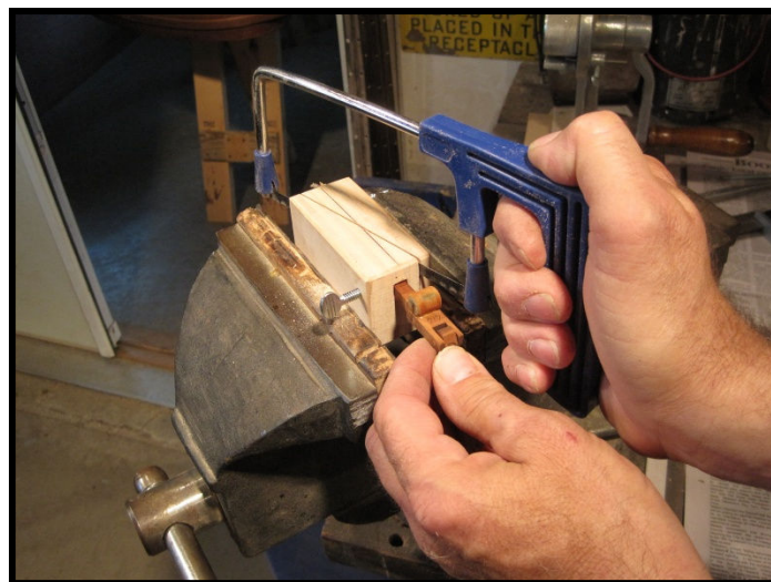
Special sawing jig required.
