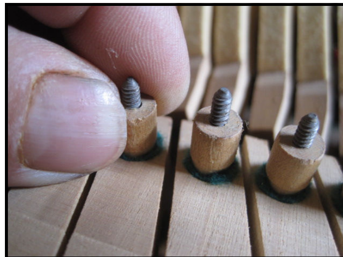
Adjusting lost motion with a fine touch.
